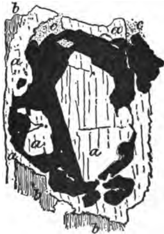
Fig. 7. Primary pyrrhotite in augite. Black, pyrrhotite; a, augite; b, urallite; c, chlorite. From W. Lindgren; 17th Annual Report United States Geological Survey, Part II.
